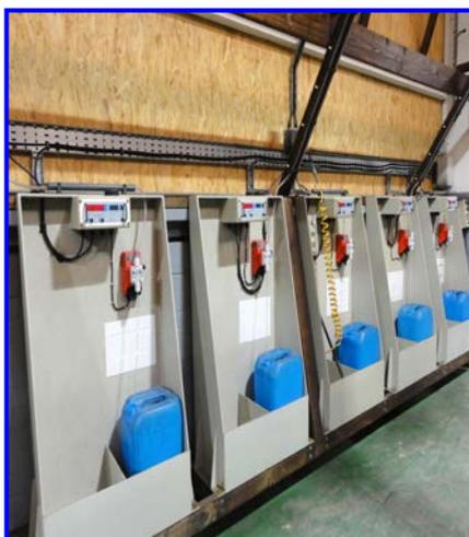
We are pleased to say that many of our customers involved in metal finishing are saving money on chemical reagents and electricity by using our model AH555 Ampere Hour meter meters to measure the current flowing through the rectifiers to a plating vessel.
