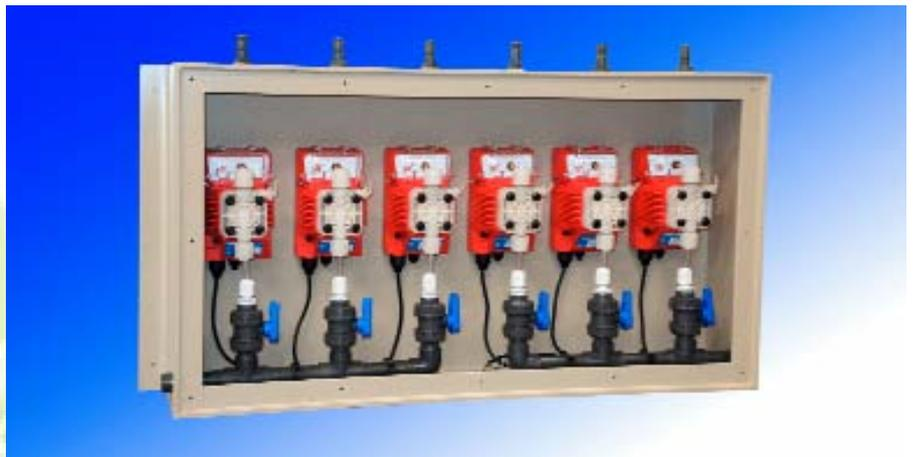
mixers from the primary chemical container and 3 assist pumps delivering to the same chemical tank, but from the secondary chemical container. This system provides an independent duty and assist dosing system. Each pump is fitted with an isolation valve and its own dosing line and injection fitting so it can be maintained without shutting the whole system down.
