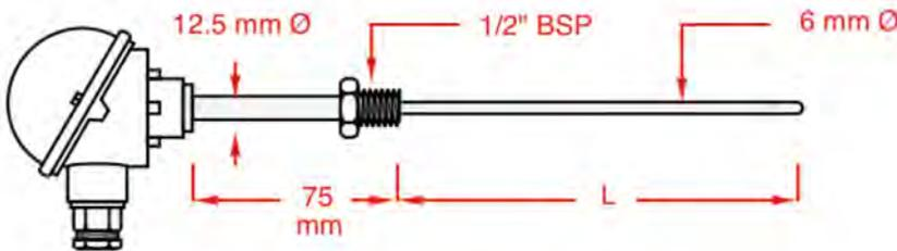
TPA-1A As above with die cast alloy connecting head usually fitted to thermocouples.
