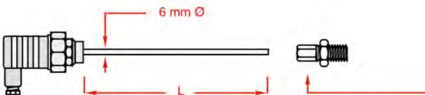
TPA- 3 Temperature probe assembly) in 316 stainless steel with Hirschmann removable connector.
