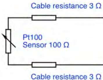
Connections for two wire instrument
