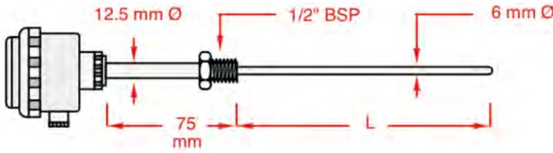
TPA-1N (Temperature probe assembly) in 316 stainless steel with ABS connecting head with terminals or optional two wire transmitter
