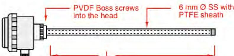
TPA-2N-PTFE temperature sensors have a 316 stainless steel shaft parallel for the whole length sheathed in PTFE with a PVDF bush so no metal parts are exposed.
