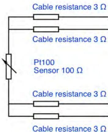
Connections for four wire instrument
