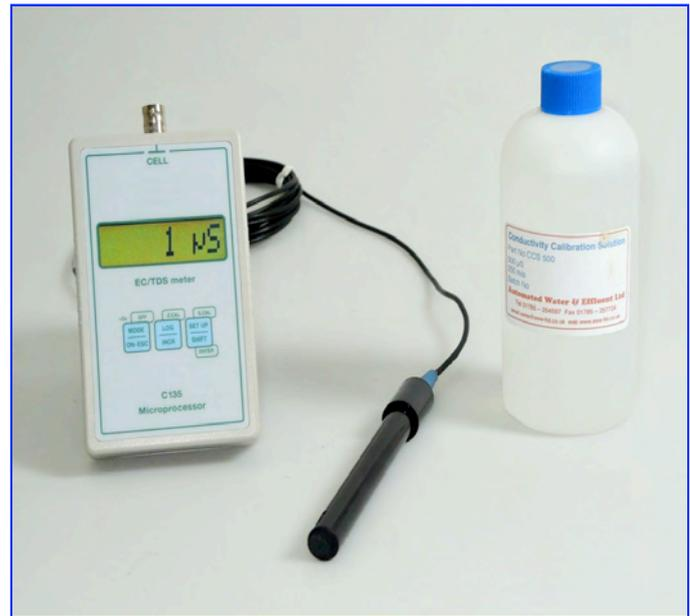
temperature / auto temperature compensation probe fitted with 900mm cable and connector, C1000 liquid calibration solution ready for use.
