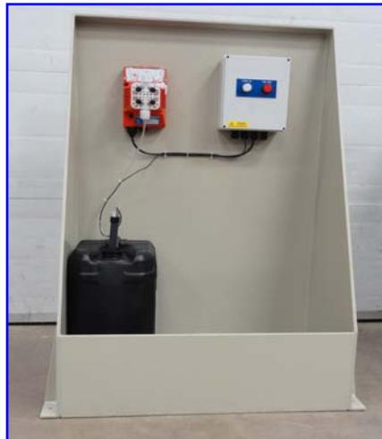
The conductivity controller controls the corrosion inhibitor pump so when fresh water is added to the system, this dilutes the chemical concentration causing the conductivity to drop. Switching on the chemical dosing pump to add chemical, increases the conductivity. The conductivity of the chemical reagent added must be considerably higher than the system solution in order for this to work.
