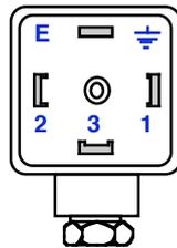
Use LMK2 cable for cells without Auto Temp Comp for cells with auto temp comp fitted used LMK4 connecting cable. The screen should be earthed at the instrument but not connected at the cell end max cable length 25 metres
