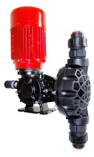
The TAM 2-4-6 series of mechanical dosing pumps are driven by an electric motor which maybe 400 volt 3 phase or optional 230 volt single phase, motors controlled by invertors are also available.
