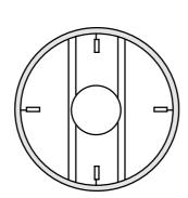
Installed with the shaft mounted vertically on the centre line of the vessel. Fitted with four strip baffles mounted vertically 90° apart with rotation clockwise when looking down the shaft so fluid is pushed down the vessel. This installation creates a turbulent fluid regime ideal for most mixing applications.
