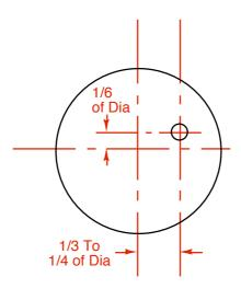
Installed with the shaft mounted vertically off centre without baffles with rotation clockwise when looking down the shaft so fluid is pushed down the vessel. The exact position depends upon the particular application and tank size. Provides good mixing without baffles. This technique places the propeller in a position which provides an acceptable flow pattern but inferior to a fully baffled tank.
