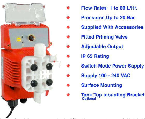
The AT-BX series of red dosing pumps are designed for either surface or foot mounting with the optional mounting bracket. The pumps outputs range from 0 - 1.5 L/Hr to 0 - 60 L/Hr and are fitted with PVC heads and ceramic ball valves with either EPDM or Viton "O" rings and seals to be specified when ordering. For greater chemical resistance when dosing concentrated reagents optional PVDF heads are available and we are able to offer PTFE ball valves.
