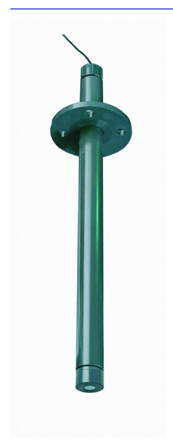
The DES1 DO2 Oxygen Electrode system is based on the Clark or Polarographic principal of measurement. Where a low voltage is applied to polarise the sensor and the current flowing through the loop is proportional to the oxygen level present. The DES1 Polarographic sensor is of simple construction easy to maintain and refurbish with new filling solution and membrane.
