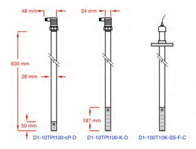
D1-10TPt100-cP-D D1 Series cell with k= 1.0 ATC by Pt100 sensor Fitted cPVC riser tube and demountable connector
