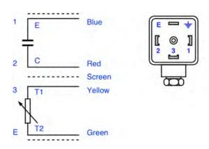
Use LMK2 cable for cells without Auto Temp Comp for cells with auto temp comp fitted used LMK4 connectiong cable. The screen should be earthed at the instrument but not connected at the cell end max cable length 25 metres
